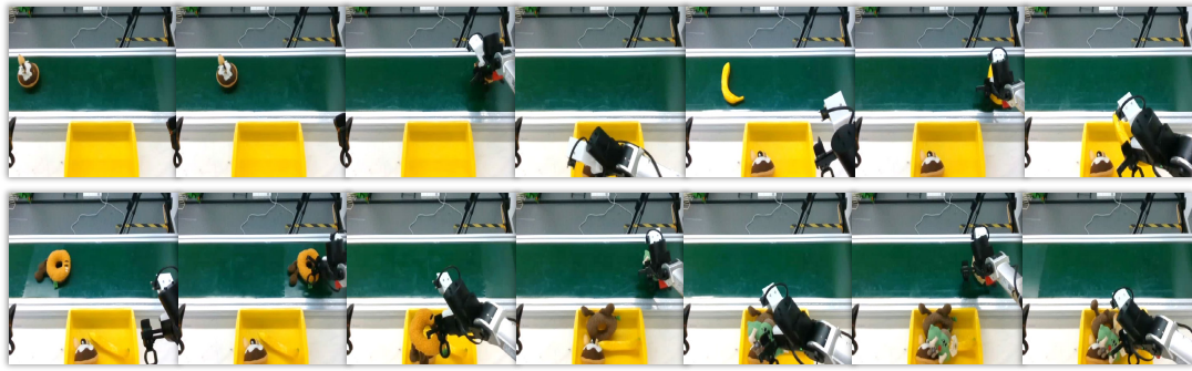
(a) Conveyor Pick (Low): continuously pick objects from the conveyor belt and place them into the box
