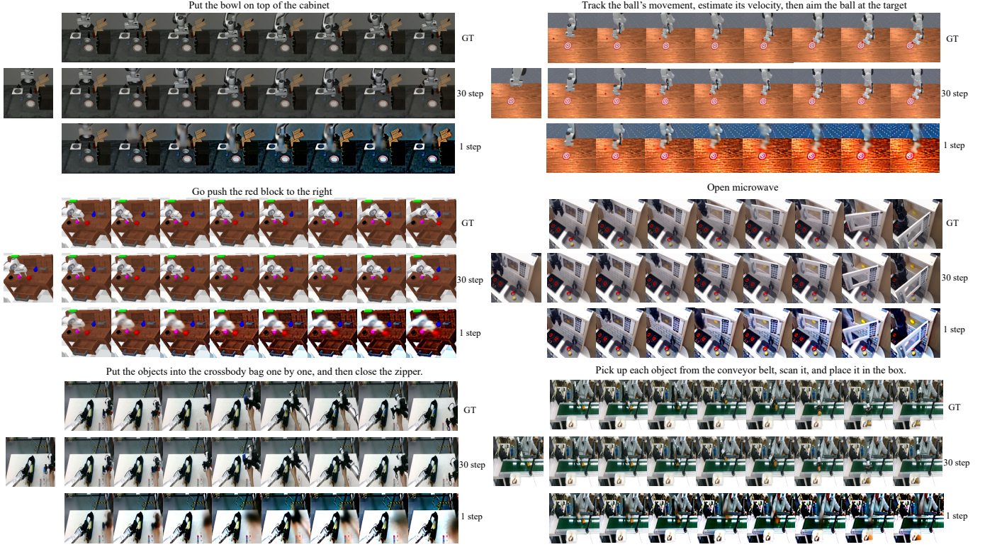
Fig. 12. Visualization of world model imagination. We compare ground-truth future observations with imagined trajectories generated using 30 and 1 denoising steps across simulation and real-world tasks, showing that the world model captures future semantic dynamics even under partial denoising.
